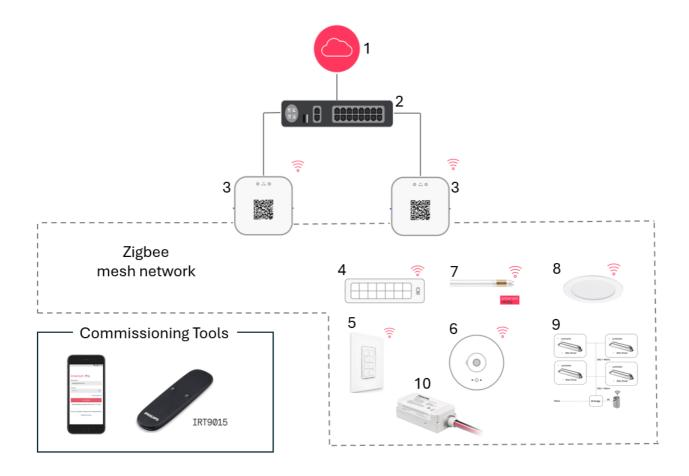
1-Interact Cloud, 2-IT infrastructure, 3-Wireless gateway, 4-Luminaires with built-in sensors/transceivers, 5-Wireless switches, 6-Battery powered ZGP sensors, 7-Smart T-LEDs, 8-Luminaires with wireless drivers, 9-DALI and 0-10V bridges with sensors/transceivers, 10-Switch relay.
