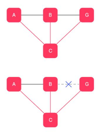
This makes the network much more robust as multiple routing paths can be used for communication.
