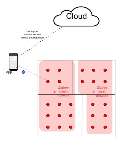
In PRF or PRA, light control is implemented using a wireless mesh network based on the Zigbee protocol: two-way communication between lights and discrete controls is solely based on this protocol. Commissioning and user control are done using a mobile phone app.
