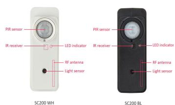
SC200 WH The IR receiver, LED indicator and RF antenna are hidden behind the plastic front cover SC200 BL The RF antenna is hidden behind the plastic front cover
