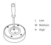
• Performing a factory reset restores sensor to un-commissioned status. Sensor is removed from current network (if any).
