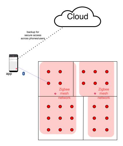
In standalone or connected, light control is implemented using a wireless mesh network based on the Zigbee protocol: two-way communication between lights and discrete controls is solely based on this protocol. Commissioning and user control are done using a mobile phone app.
