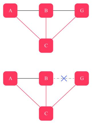
Zigbee routing between wireless devices
