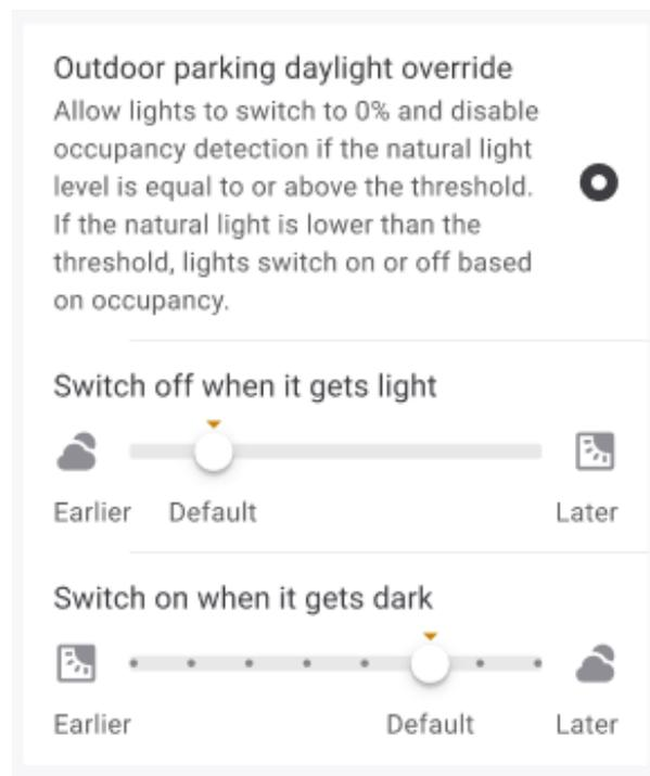
Switch off when it gets light: This parameter will configure the light level threshold at which the sensor will switch off the lights in the evening. Always use the default value as a starting point. If the lights are switching off too late or too early, slightly adjust the slider to the opposite direction. For example, if lights are switching off too early in the morning, move the slider to the "Later" side and check again.
