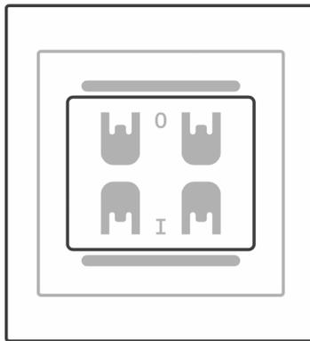
When you click back the rocker, look at the back and make sure that the side with the two plastic knobs is at the right hand side when clicked back to the wireless module.
