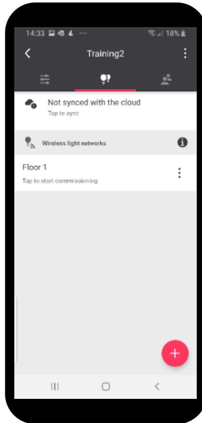
As an example, the screenshot above shows what to expect after creating a light network called **Floor 1**. It also displays an important message *Not synced with the cloud*. Next to unlocking the project (which automatically triggers a sync), it is important that a backup is created of the most crucial credentials of the project. This allows for
