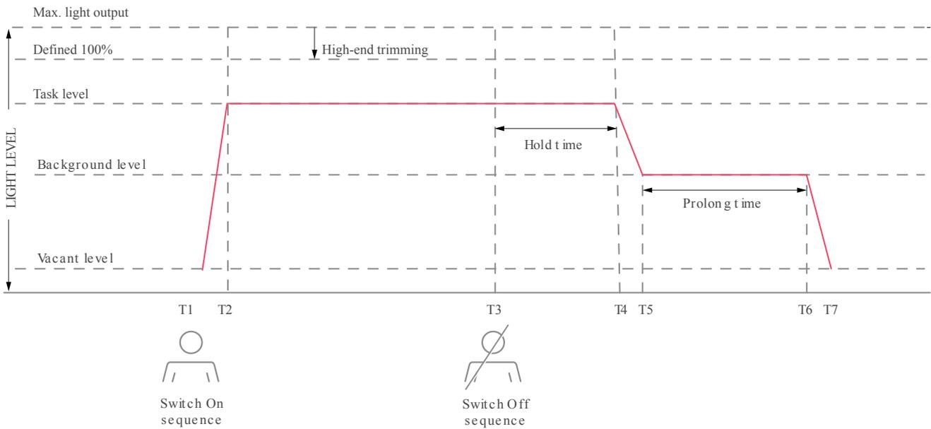
When occupancy is detected by one of the sensors in the group, the lights in the group go from *vacant level* to *task level* (T1 → T2).<sup>[2]</sup> When no occupancy is detected anymore by one of the sensors, the *hold time* period starts (T3). Upon expiration of the hold time, the lights are dimmed down to the *background level* (T4 → T5) and remains at this level for the duration of the *prolong time*. Upon expiration of the prolong time, the lights dim down to *vacant level* (T6 → T7).
